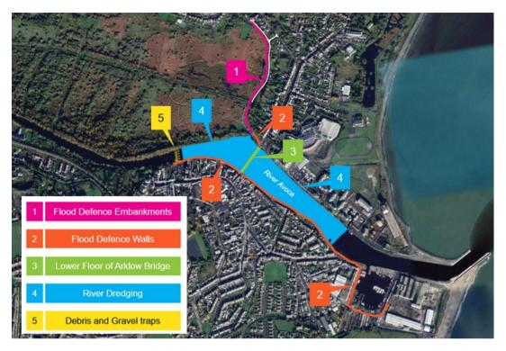
Figure 4.1: Overall Layout of Proposed Flood Relief Works
